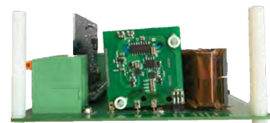
Side views of the proposed high power density online UPS prototype built in the lab, capable of achieving a power density of 26.4 W/in 3 . Image provided.
